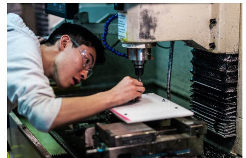
James Jiao (sr.) changing the cutter on the CNC mill while machining a part for the elevator.
