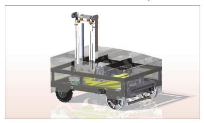
This machine of metal, plastic, and semiconductors is a fast and versatile robot with a multistage lift that has the ability to elevate the robot on any piece of sturdy metal bar up to seven feet high. A strong kicker and controlling roller makes this machine a potent soccer player.
