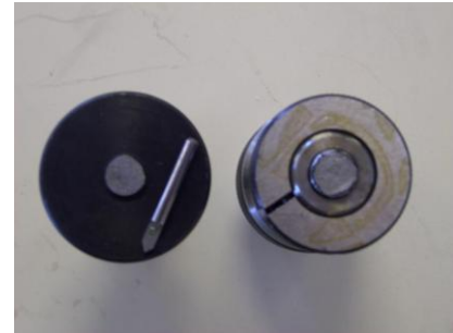
Figure 4. Even the side loads from a small engraving tool can catastrophically damage the Jacob's Taper
