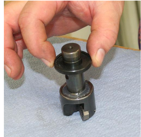
Figure 17. Place the conversion ring on the tool
