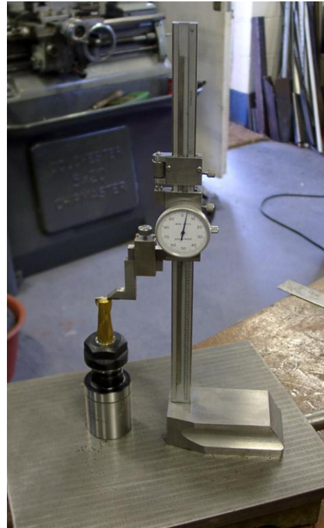
Figure 2. Touching off tools on a surface plate, using the TTS measurement fixture to support the ground precision ring.
