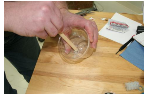
Figure 15. Mix the epoxy. Avoid skin contact
