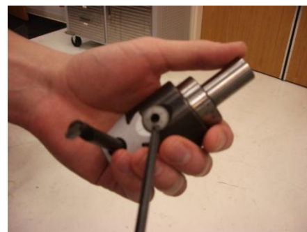
Figure 6. Adjusting the boring head
