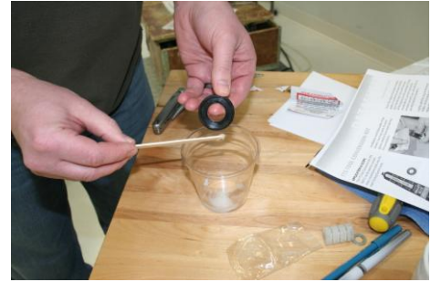
Figure 16. Spread the Epoxy on the conversion ring
