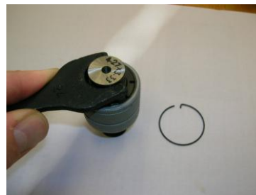
Figure 11. Once the spring clip has been removed, the spanner can be used to tighten or loosen the adjustable nut.
