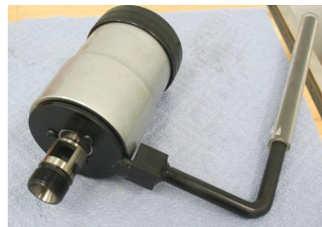
Figure 7. Reversing Tapping Head with Brake Rod installed.
