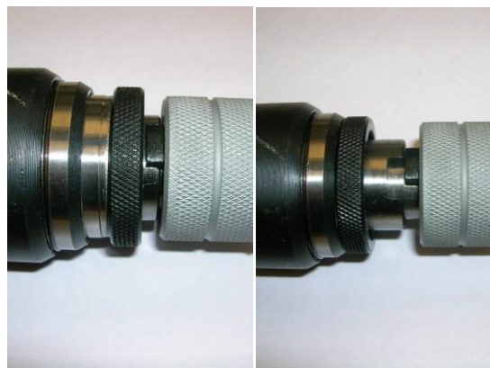
Figure 10. To install the collet into the tapping head, press firmly and twist until teeth engage and the collar snaps in place.
