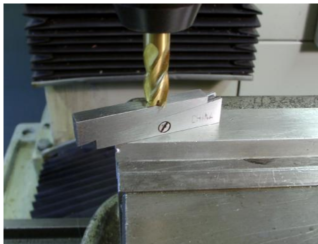
Figure 6.14 – Parallel adjusted to gap
