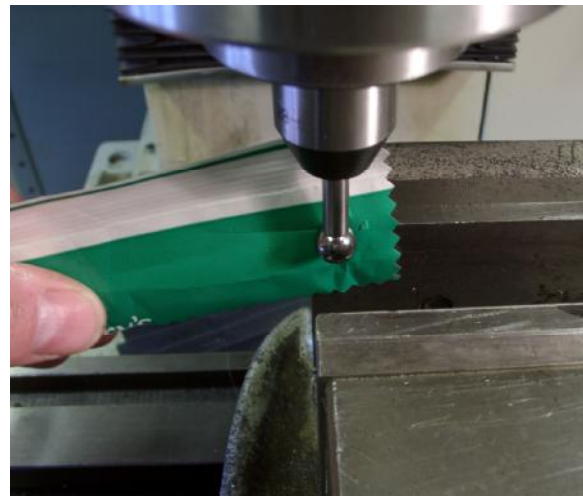
Figure 6.22 – Measuring vise jaw Y position
