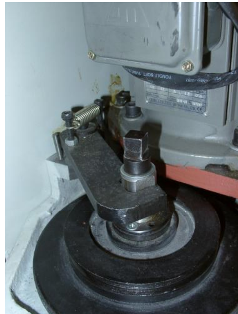
Figure 5.7 – Spindle lock fork engaged
