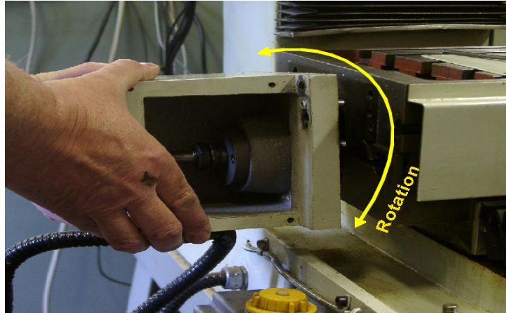
Figure 9.6 – Feeling preload in bearings
