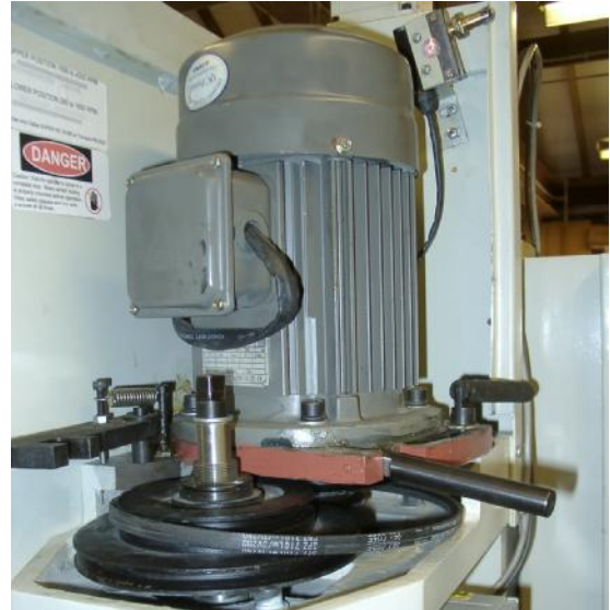
Figure 5.8 – Changing spindle speed range
