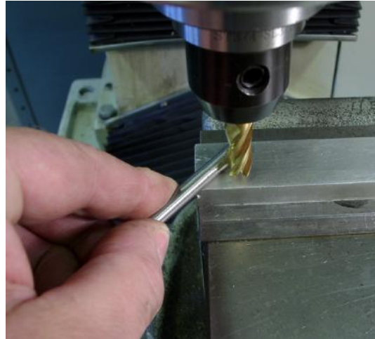
Figure 6.12 – Tool much too low for gauge
