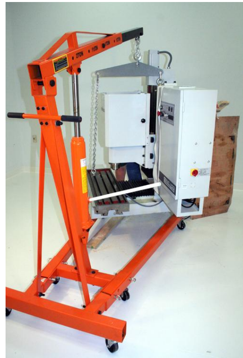
Figure 2.7 – Hoist bar for slinging the mill
