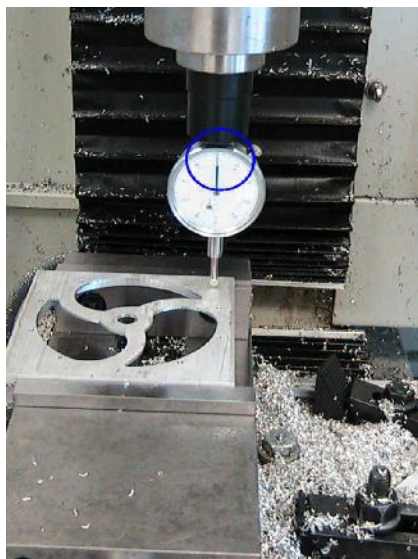
Figure 6.7 – Dial zero touching work
