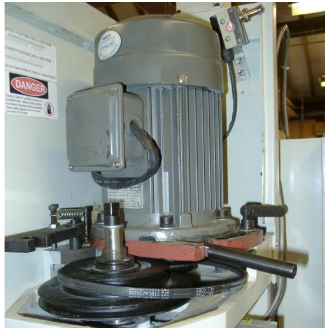
Figure 2.17 – Changing spindle pulleys
