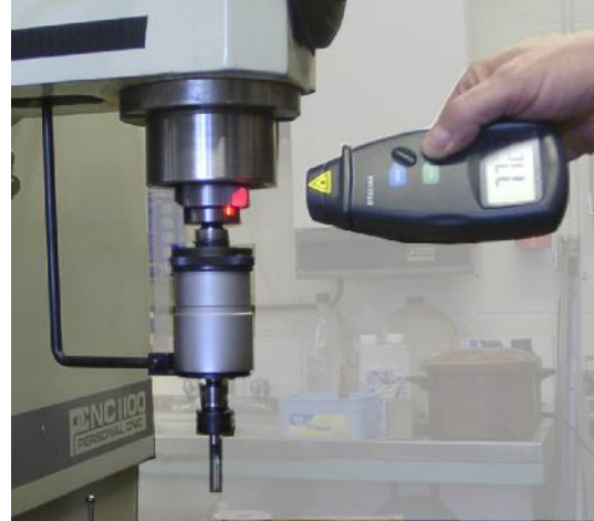
Figure 8.27 – Measuring spindle speed
