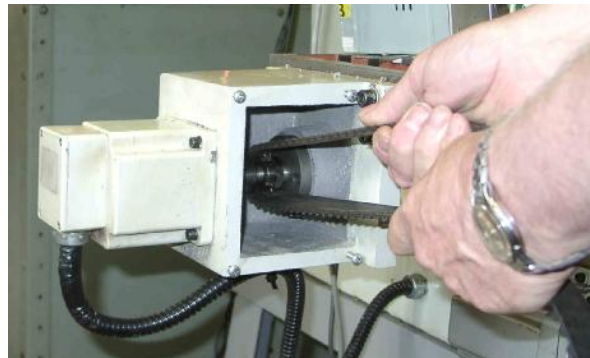
Figure 2.9 – Manual moving table by back of old toothed belt
