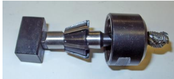
Figure 8.24 – Tap collet and anti-rotation block
