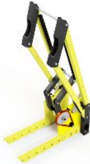
The final model of the shooter arms and crank gearbox, with counterbalancing.
