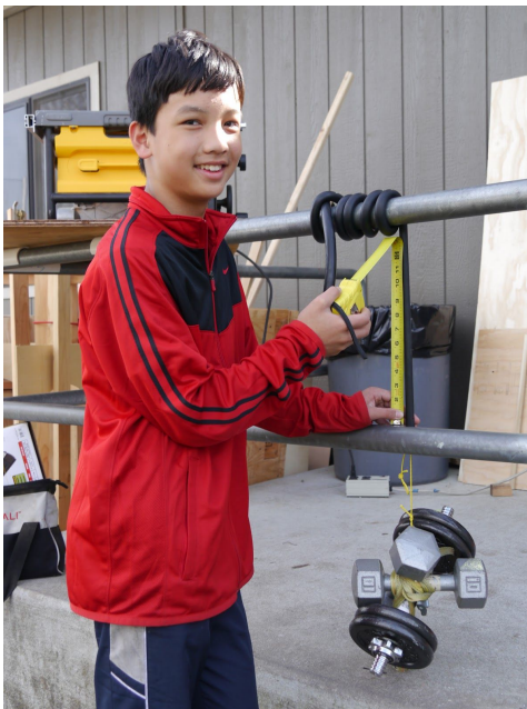
Left: Measuring the spring constant of 3/4" latex rubber tubing with 43 lbs of weights. Andrew Ng (Freshman).
