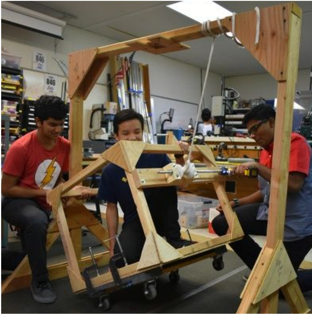
Sophomores Shreyas Mohidekar (Left), Andrew Ng (Center), and Atul Nair (Right) test the velcro winch on a mockup of the robot.
