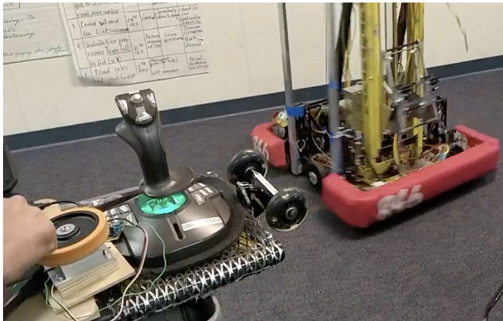
An absolute steering wheel prototype controlling the robot's angle.
