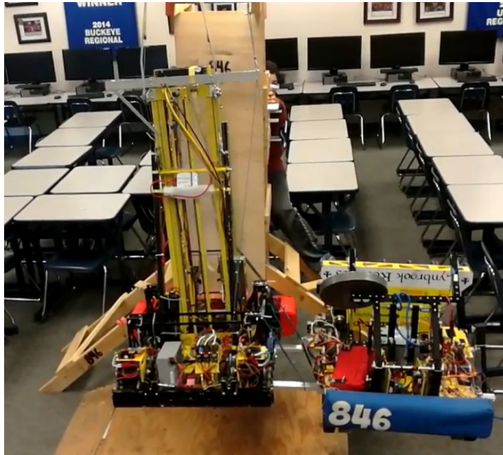
"Wes" lifts a retired robot, with weights added to make it 145 pounds.
